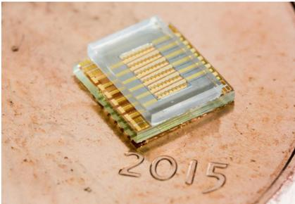
**Fig. 1:** Menlo Microsystems’ 6-Channel, 25W per channel, SPST RF MEMS switch. This combination of glass and metal enables highly broadband RF switches.
