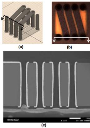
**Fig. 6:** 3D TGV inductor structure (a) 3D rendering, (b) top-down photograph (c) cross-sectional SEM of TGV with conformal Cu plating on the TGV sidewalls, and the top and bottom sides of the glass to form a 3D TGV inductor.
