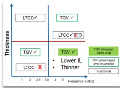
**Fig. 7:** The properties of glass make it well-suited for RF devices with excellent high frequency performance.
