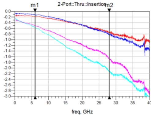
**Fig. 3:** Insertion loss of two Menlo Microsystems RF MEMS SPST switch designs on both glass (top two traces) and high resistivity silicon (bottom two traces). The glass based performance is 0.8 dB vs. 1.7 dB for Si at 28GHz in frequency.
