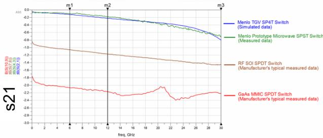
**Fig. 5:** Broadband performance of RF MEMS-based switch has been demonstrated to outperform other technologies. Source: Menlo Microsystems.
