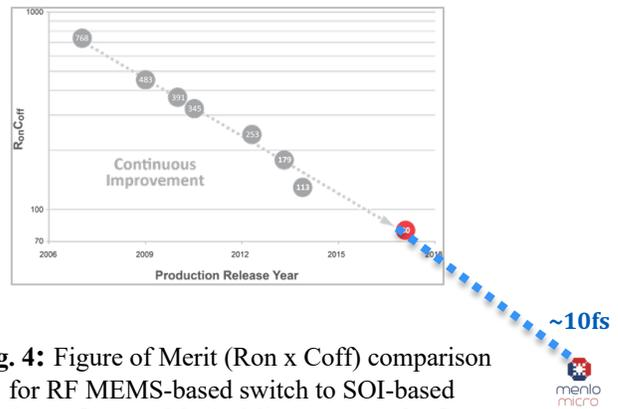
**Fig. 4:** Figure of Merit (Ron x Coff) comparison for RF MEMS-based switch to SOI-based products. Source: Menlo Microsystems & pSemi
