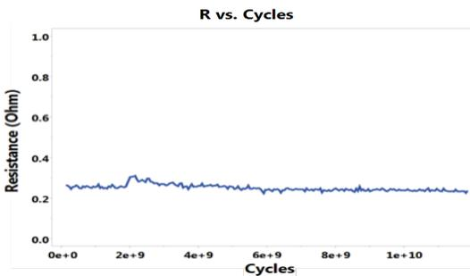
**Fig. 2:** Typical Resistance of 6-Channel 48-cantilever MEMS switch from Menlo Microsystems
