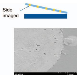
**Figure 13:** SEM image of bottom of metallized via after de-bond (no polishing).
