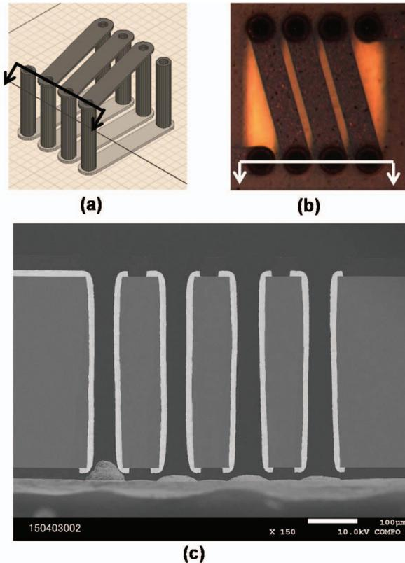
**Figure 4:** 3D TGV inductor formation. (a) 3D rendering, (b) top-down photograph, (c) cross-sectional SEM of TGV with conformal Cu plating on the TGV sidewalls and the top & bottom sides of the glass to form a 3D TGV inductor
