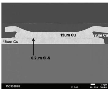
**Figure 5:** Cross-sectional SEM of TGV with conformal Cu plating on the TGV sidewalls and the top & bottom sides of the glass to form a 3D TGV inductor.
