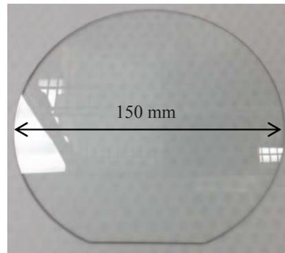
**Figure 11:** Image 100 um thick glass with 30 um diameter vias temporarily bonded onto a glass carrier using ALoT technology.
