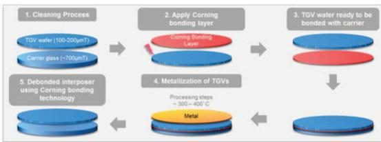
**Figure 9:** Schematic showing an approach for handling thin glass through metallization.
