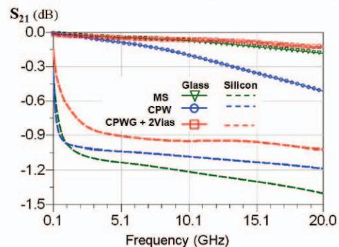
**Figure 3:** The insertion loss ( $S_{21}$ ) from transmission lines on glass and standard silicon substrates showing much less loss in glass at higher frequencies.
