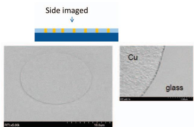
**Figure 12:** SEM of vias on top surface after planarization.
