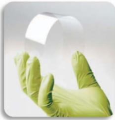
**Figure 8:** Manufacture of high quality ultra-slim flexible Corning® Willow® Glass provides substantial opportunities to deliver substrates for TGV that do not require post processing.
