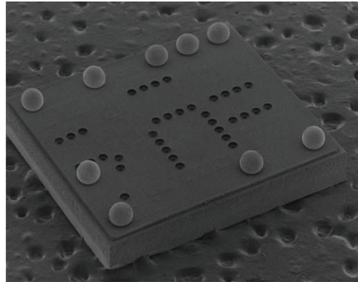
**Figure 6:** SEM bird's eye view of completed LC networks device.
